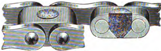
FIG. 393.—The Duryea Self-oiling Sprocket Drive Chain. The body of each link is bored out as shown, and a plug of felt inserted in the opening. The felt absorbs oil readily, at once thoroughly lubricating the moving parts and increasing the tightness of its own adhesion. This feature insures a noiseless chain.
